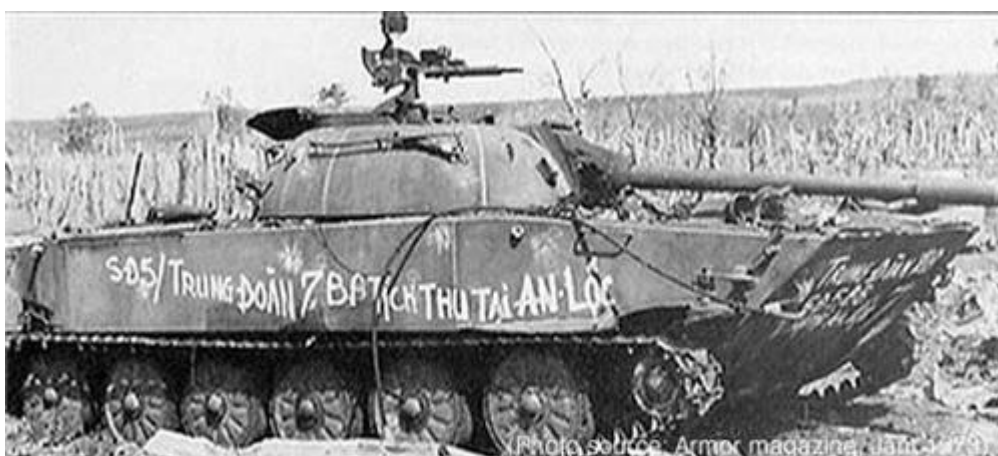
This PT76 was destroyed by M72 fire. The lettering reads: Confiscated at An Loc by 7th Regiment/5th Infantry Division
